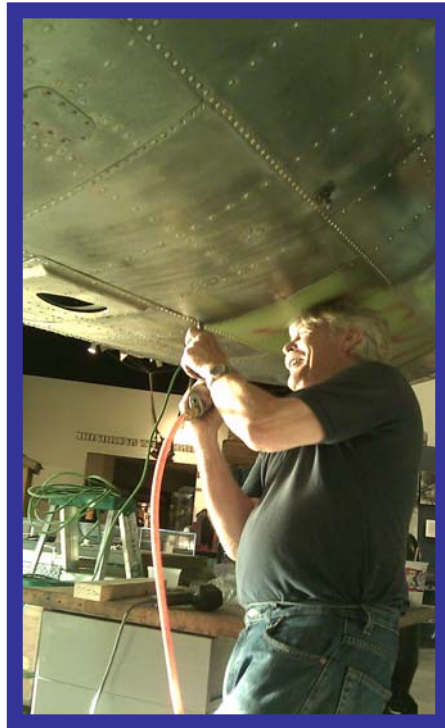
Jack Nilsen hard at work riveting the new skin panels under the nose
