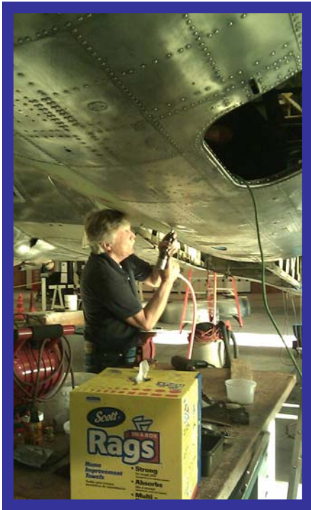
Jack Nilsen hard at work riveting the new skin panels under the nose
