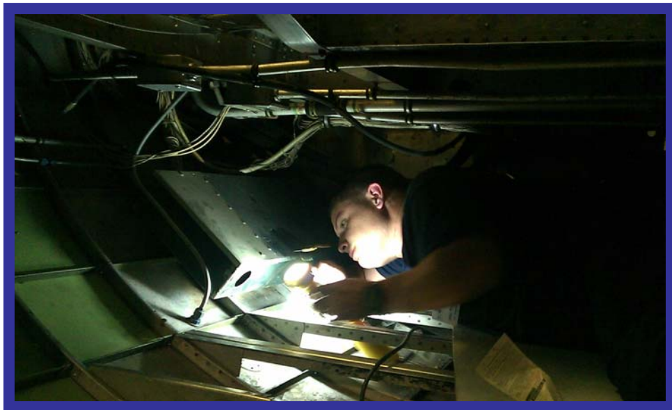
Volunteer John Finch checking new aluminum sheeting under the cockpit floor
